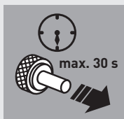
Fig. 3d: Waiting and releasing the throttle knob
