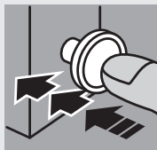
Fig. 3b: Pressing the gas valve knob
